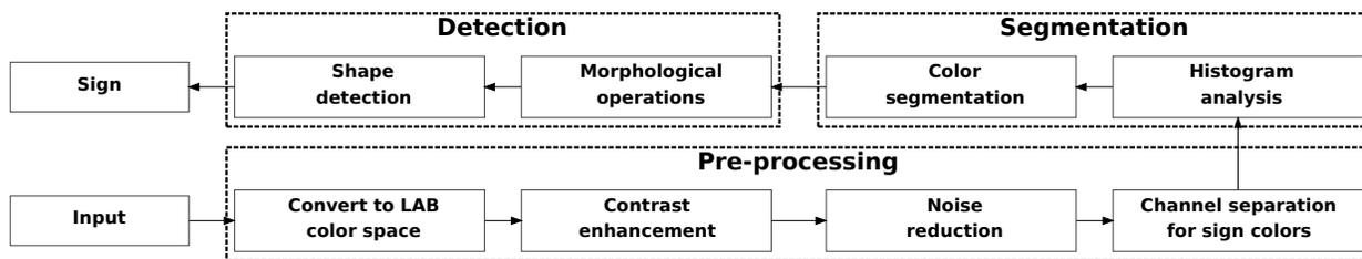
Figure 2. Proposed Traffic Sign Detection method.
