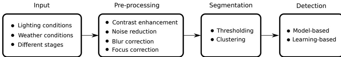
Figure 1. General Traffic Sign Detection system
