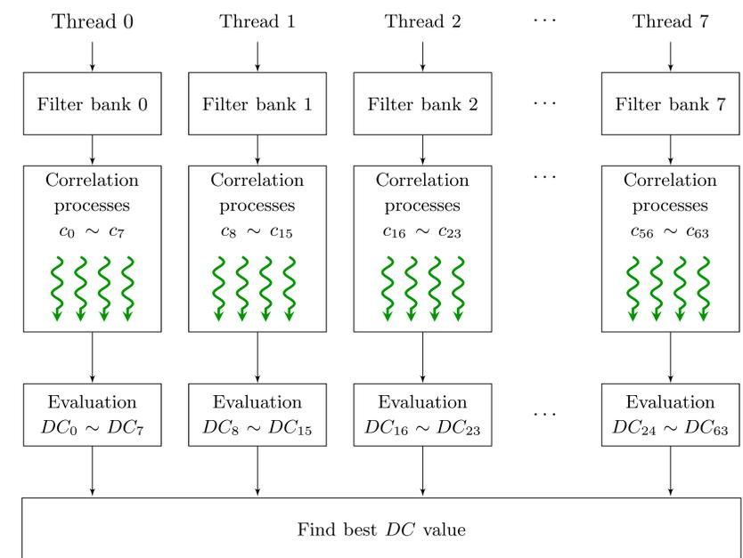
Figure 3: Parallel implementation using OpenMP and CUDA CUFFT.
