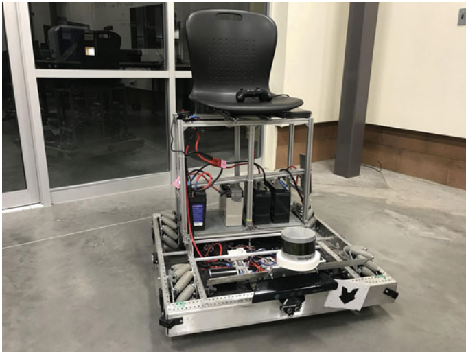
Fig. 15.39 Autonomous vehicle scale prototype [58]
