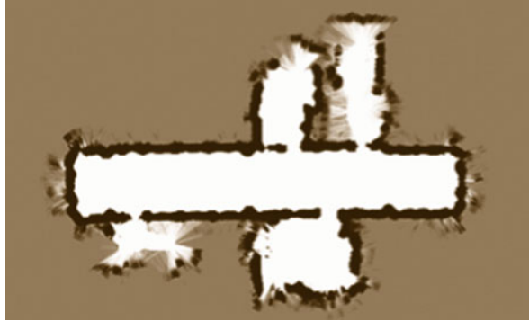
Fig. 15.17 Occupancy grid map obtained from ultrasound data [33]
