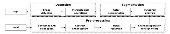
Figure 2. Proposed Traffic Sign Detection method.
