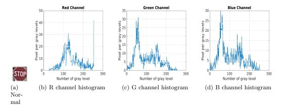
Figure 4. Distributions of each RGB channel of red sign with normal condition.
